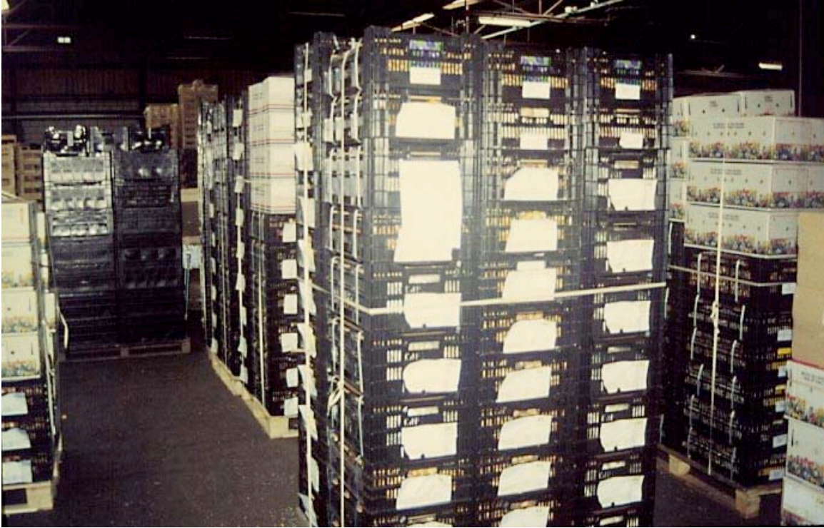
Pallets of bulbs ready for loading into a reefer container. The perforated sides of the plastic shipping crates allow air movement through the mass of bulbs on the pallet.
