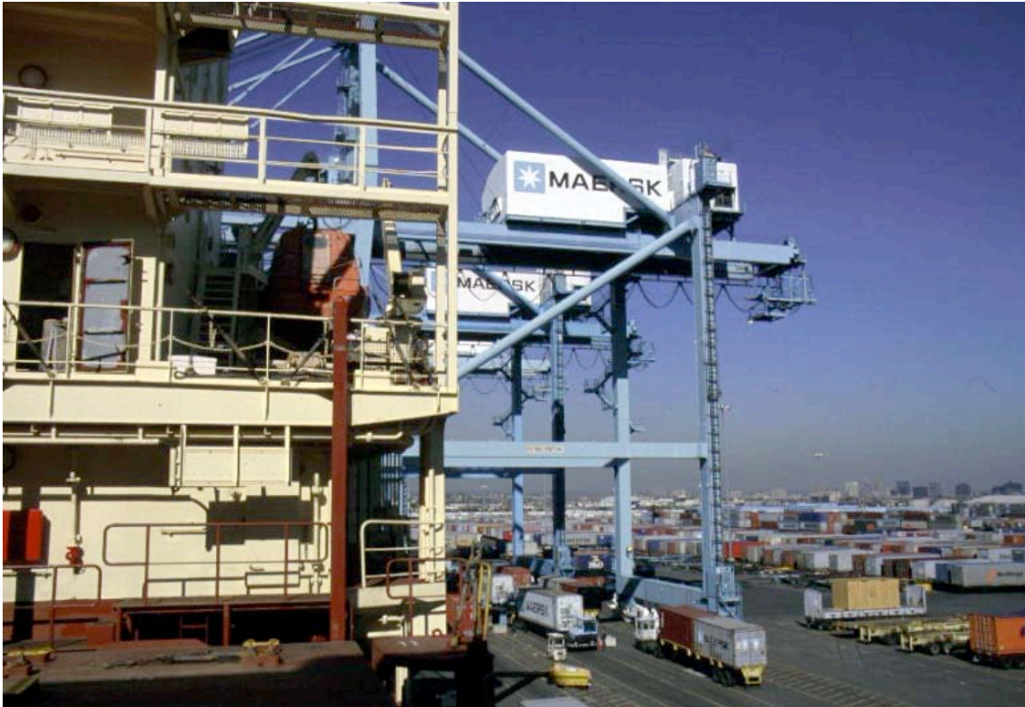
View from aboard a container vessel during unloading in port. As each container is removed from the ship, it is placed on a dolly for transport within the arrival area.
